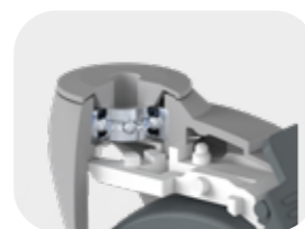
Section Picture: Swivel Head with Ball Bearing
